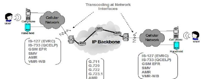
Figure 1. Tandem Voice Coding in Mobile-to-Mobile Calls
