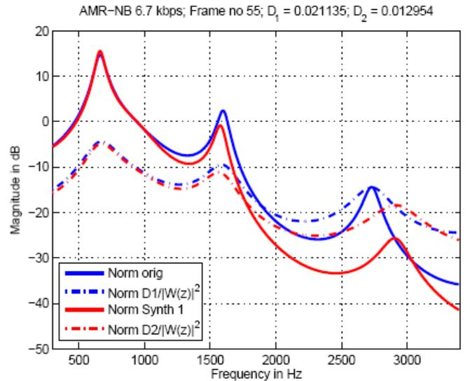
Figure 6. Normalized Spectra for Two Stage Tandem Coding with AMR-NB at 6.7 kbps
