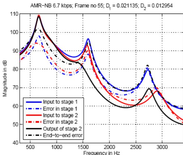
Figure 3. Spectra for Two Stage Tandem Coding with AMR-NB at 6.7 kbps
