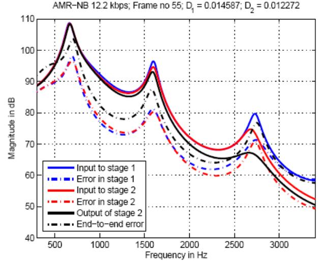
Figure 5. Spectra for Two Stage Tandem Coding with AMR-NB at 12.2 kbps
