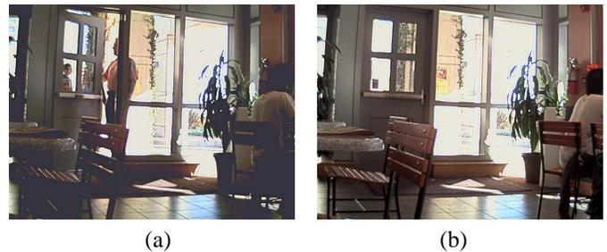
Fig. 1. (a) Low dynamic range frame captured by traditional auto-exposure (b) High dynamic range (HDR) frame created using the alternating exposure technique — note improved clarity and details in the foreground.
