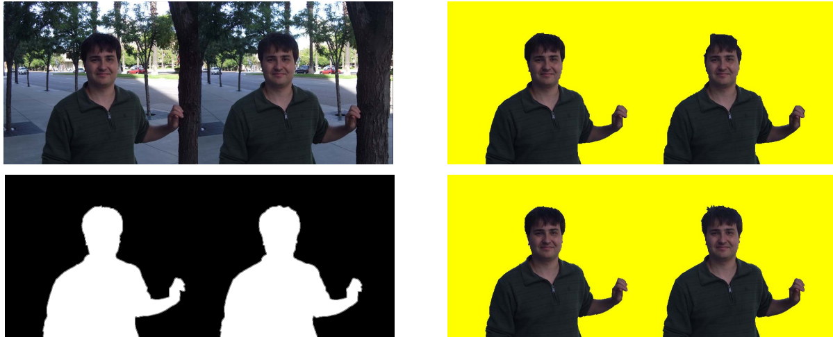
Fig. 4. A successful case. Left top : Input stereo pair. Left bottom : ground truth segmentation. Right top : Result of Consistent Delta proposed by [3]. Right bottom : our result. The hair of the person is better extracted in our result.
