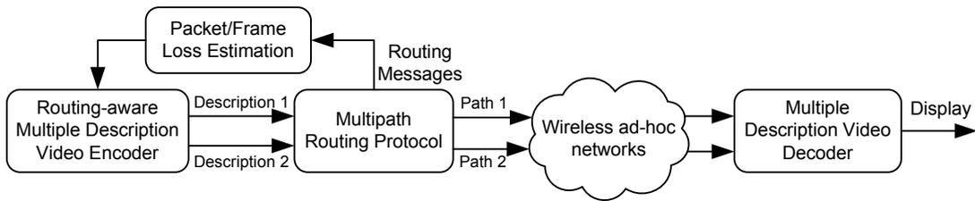
Fig. 1. System architecture of the proposed system using routing-aware multiple description coding and multipath routing
