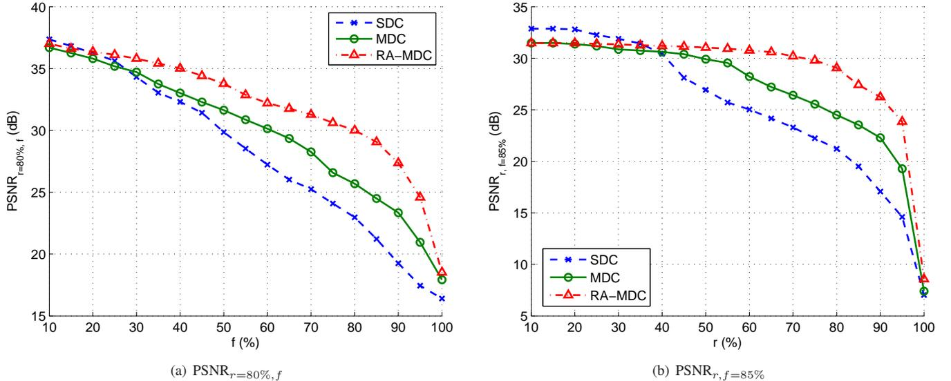
Fig. 5. Comparing  $PSNR_{r,f}$  of SDC, MDC, and RA-MDC. Foreman sequence (CIF, 15fps) at 400 kbps, packet loss rate 4.5%. Average PSNRs of SDC, MDC, and RA-MDC are 32.20 dB, 32.45 dB, and 33.51 dB respectively
