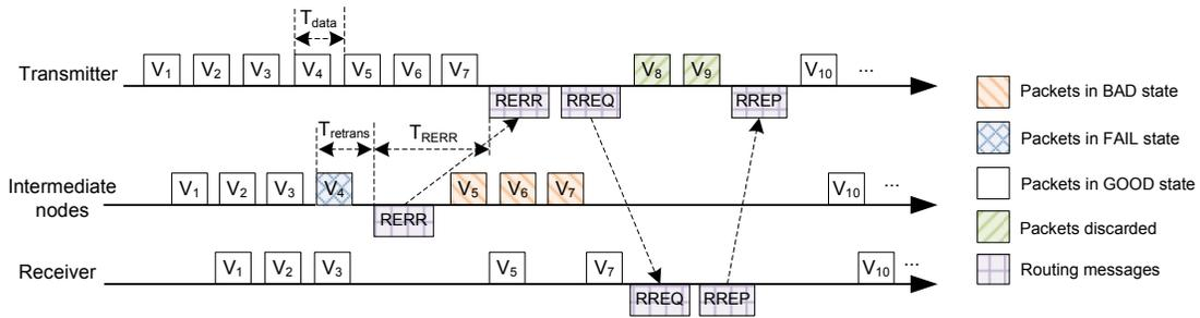
Fig. 1. An example to illustrate the packet losses in the network and the corresponding routing messages
