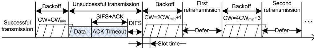
Fig. 2. Packet retransmission procedure based on basic access mechanism
