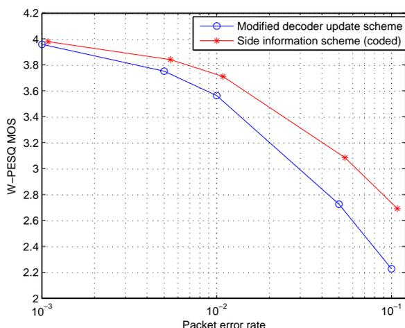
Figure 14. Performance comparison for packets with and without side information
