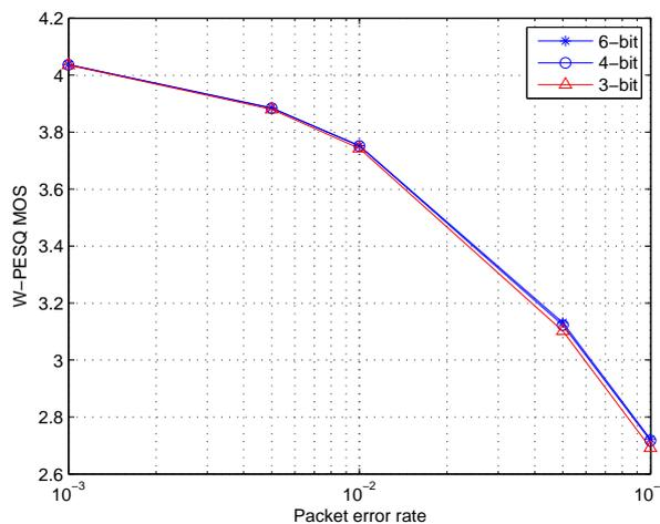
Figure 8. Performance of coded side information scheme under different quantization levels used for encoding the past reconstructed and difference signals
