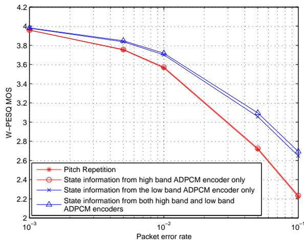
Figure 4. Performance comparison of G.722 PLC with various state information for individual subbands without pitch side information
