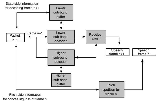
Figure 13. Decoding of the  $n^{th}$  and  $n + 1^{th}$  frame when the  $n^{th}$  frame is lost, for the side information based scheme
