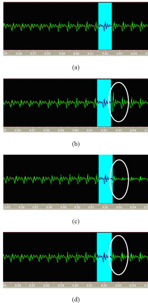
Figure 1. Waveforms for a) Reference decoded speech (no loss), b) Speech decoded using pitch repetition c) Speech decoded using the decoder update scheme d) Speech decoded using the Modified Decoder update scheme. The highlighted portion represents the lost frame, and the circled portion represents the correctly received frame following the lost frame
