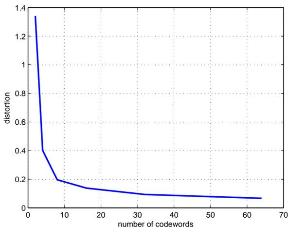
Figure 7. Codebook sizes and corresponding distortion in VQ design for zero coefficients and scaling factor
