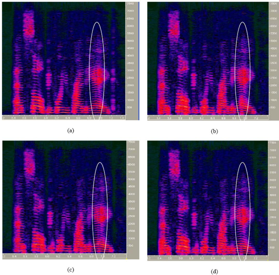
Figure 2. Spectrograms for a) Reference decoded speech (no loss) b) Speech decoded using pitch repetition c) Speech decoded using the decoder update scheme d) Speech decoded using the Modified Decoder update scheme. The circled region indicates the part of the spectrogram corresponding to the portion of the speech waveform shown in Fig. 1.
