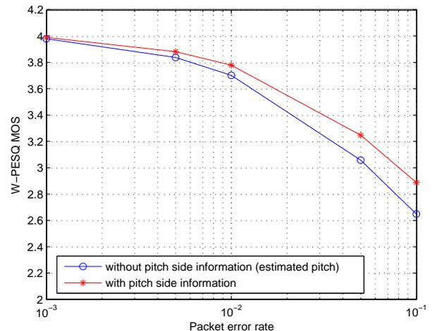
Figure 5. Performance comparison of Side Information based scheme with and without accurate pitch information.
