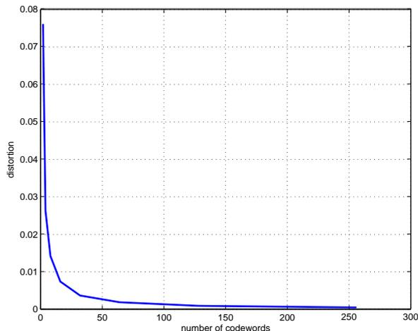
Figure 6. Codebook sizes and corresponding distortion in VQ design for LSF coefficients
