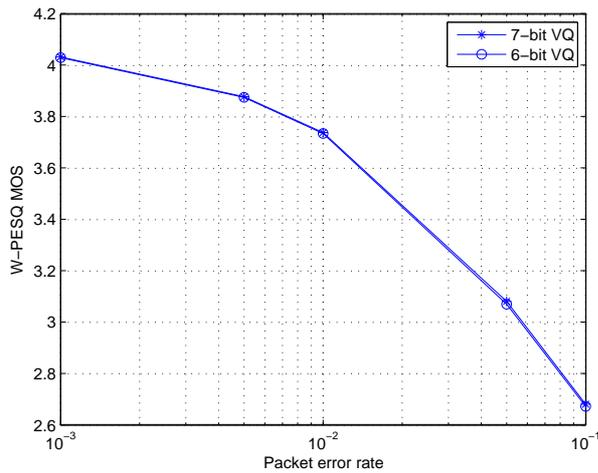
Figure 9. Performance of coded side information scheme under different quantization levels used for encoding the LSF coefficients
