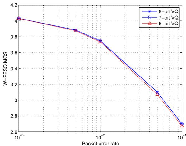
Figure 10. Performance of coded side information scheme under different quantization levels used for encoding the zero coefficients and the scaling factor
