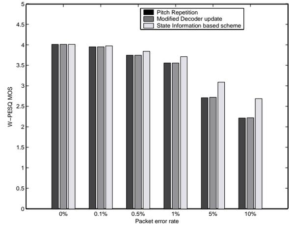
Figure 3. Performance of G.722 PLC using 1) Pitch repetition 2) Modified decoder update + pitch repetition 3) State side information + pitch repetition, all with estimated pitch
