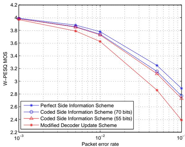
Figure 11. Performance comparison of the modified decoder update scheme and the side information scheme with perfect side information and coded side information using 70 bits and 55 bits
