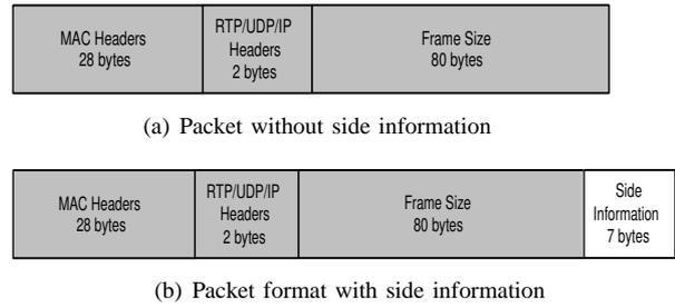
Figure 12. Packet format for 802.11a voice packet using Robust Header Compression (RoHC) with and without side information
