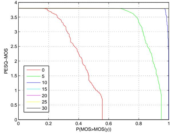
Fig. 6. CCDF for 20ms G.729 payload sizes at 6 Mbps for different SNRs in frequency selective multipath fading
