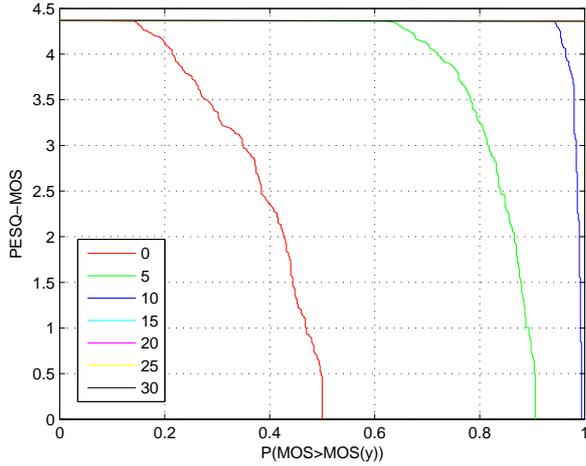
Fig. 4. CCDF for 10ms G.711 payload sizes at 6 Mbps for different SNRs in frequency selective multipath fading
