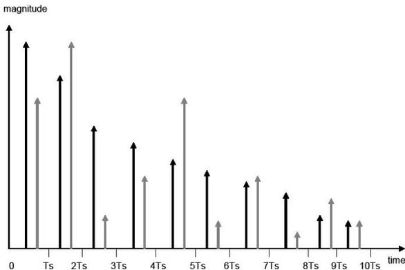
Fig. 1. Multipath channel impulse response showing average response (black) and an individual realization (grey)
