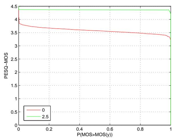
Fig. 7. CCDF for 10ms G.711 payload sizes at 6 Mbps for different SNRs in AWGN only channel
