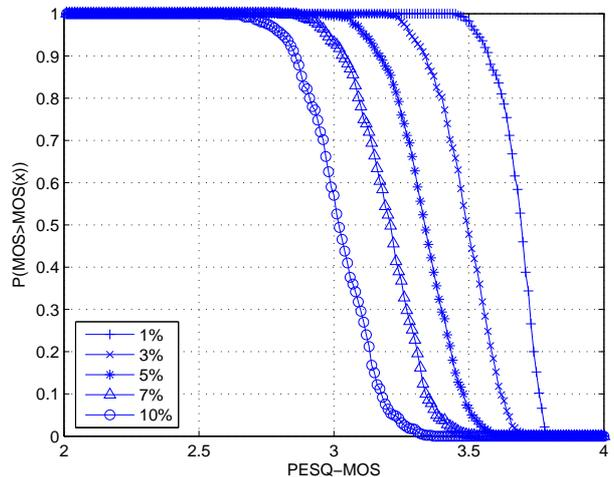
Fig. 2. CCDF of PESQ MOS values for G.729 coded speech with frame size of 10ms for different PLR
