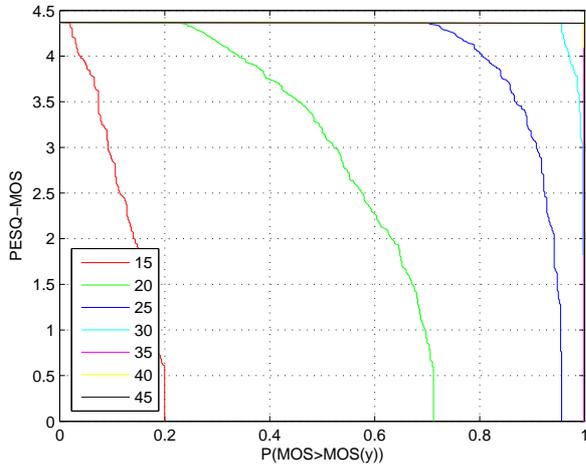
Fig. 5. CCDF for 10ms G.711 payload sizes at 54 Mbps for different SNRs in frequency selective multipath fading
