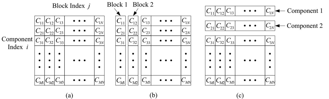
Fig. 1. Encoding transform coefficients. (a) Coefficients of  $N$  blocks, (b) Encoding block by block, (c) Encoding component by component.
